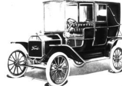
6-Passenger Town Car, Equipped with 3 Oil Lamps, Tubular Horn and Kit of Tools
